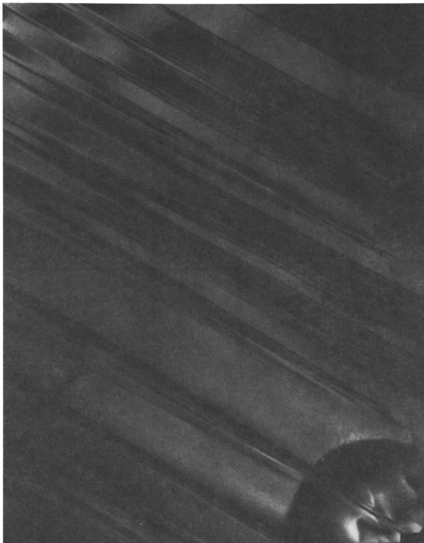
Figure 3. Transmission electron micrograph showing planar defects in \text{YBa}_2\text{Cu}_3\text{O}_7 uniformly spaced about 2000\text{\AA} and dispersed in the specimens. These have been identified as twins formed because of the slight difference in the a and b axes.
